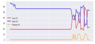
All of the sensor data is preprocessed into a single channel and the graph shows that data. When fames are simulated are in the environmnet at few particular instants, the(yellow) levels hike. At the same particular point there is huge change observed in the tempereture as well as in the humidity levels in the environment.
