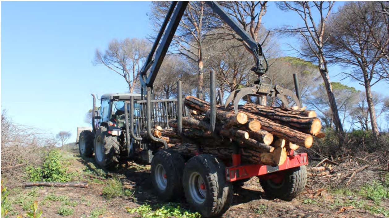
FIGURA 6. Clearing on road by tractor and light self-loading trailer. Image: P. Pons.
