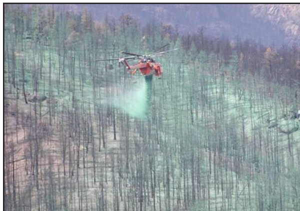
Figure 4. BAER hillslope treatments to reduce erosion: (top) log erosion barriers, (middle) aerial seeding, and (bottom) hydro mulching. (Photos by Peter R. Robichaud.)
