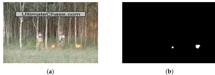
Figure 7. The smallest fire blob that can be detected by our model with area of 20 pixels. (a) Original image; (b) detected small fire blob.
